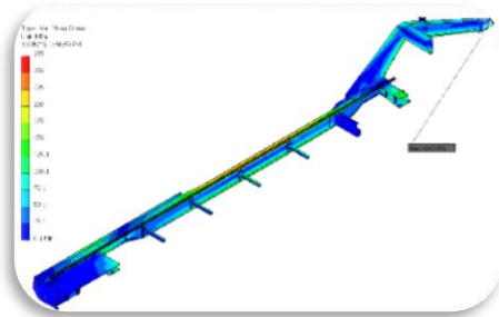
Rollingstock chassis life analysis – TLM, HOSN Wagon
